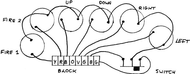
The keytops are assembled and fixed as shown below. The joyboard can be tested by using the short program below, which prints out two columns of numbers which should change when keys are pressed. If it works with the switch in one position, try it in the other and the other column should change. If both change at the same time, check the connections on the slide switch. The numbers are :- Left 4, Right 8, Up 1, Down 2, Fire 1 32, Fire 2, 16.
